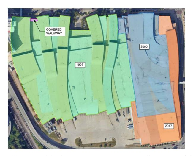
Following a successful roof replacement project at Nationwide Arena, the FCCFA is particularly interested in the use of a liquid applied roofing membrane for this project. The liquid applied membrane will reduce the need for significant tear-off and thus minimize impact on GCCC operations. The selected firm shall consider solutions capable of imitating the current roof colors and design aesthetic.
